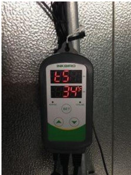
Adjust the Heating Differential HD value on the INKBIRD to 2°F/1°C following the instructions on the INKBIRD manual.
