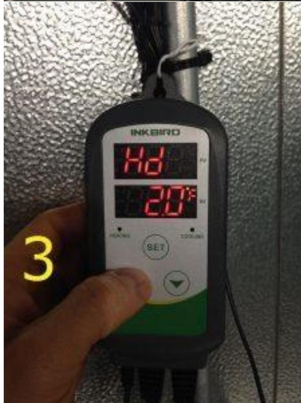
Plug your heater in the receptacle labeled HEATING on the INKBIRD plug in cord.
