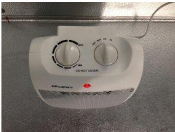
**NOTE:** Heaters are very efficient. A small heater can handle large rooms. As a general rule, you need a heater that has (Area X 10) in watts power. For example, a 100 sq ft room would require a 1000W heater. **If your heater is a 1200W or a 1500W, run your heater on Medium or Low (DO NOT RUN ON HIGH as the InkBird cord won't be able to handle the load of the Heater).**
